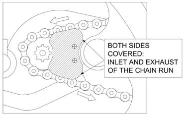
Figure 4 : Front sprocket protection
