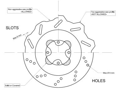
Figure 7 : Rear brake disk holes
