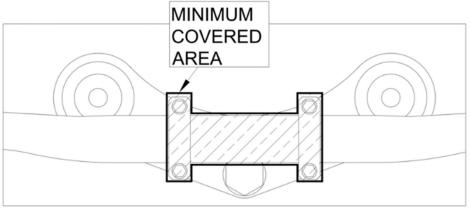
Figure 2 : Handlebar covering
