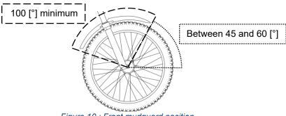
Figure 10 : Front mudguard position
